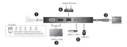
1. Plug in the power adapter to the USB-C DC in Port on your UH3236.
